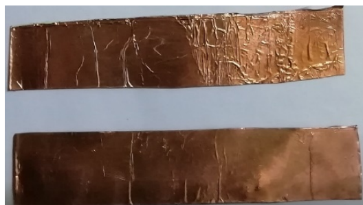
Figure 15: Copper tape electrode for measuring transverse and through thickness resistance
