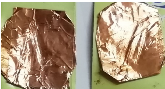
Figure 14: Copper tape electrode measuring longitudinal resistance
